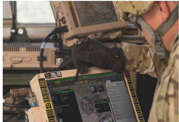
Joint Battle Command-Platform (JBC-P) is the Army's next-generation friendly force tracking system, equipping Soldiers with a faster satellite network, secure data encryption and advanced logistics.
